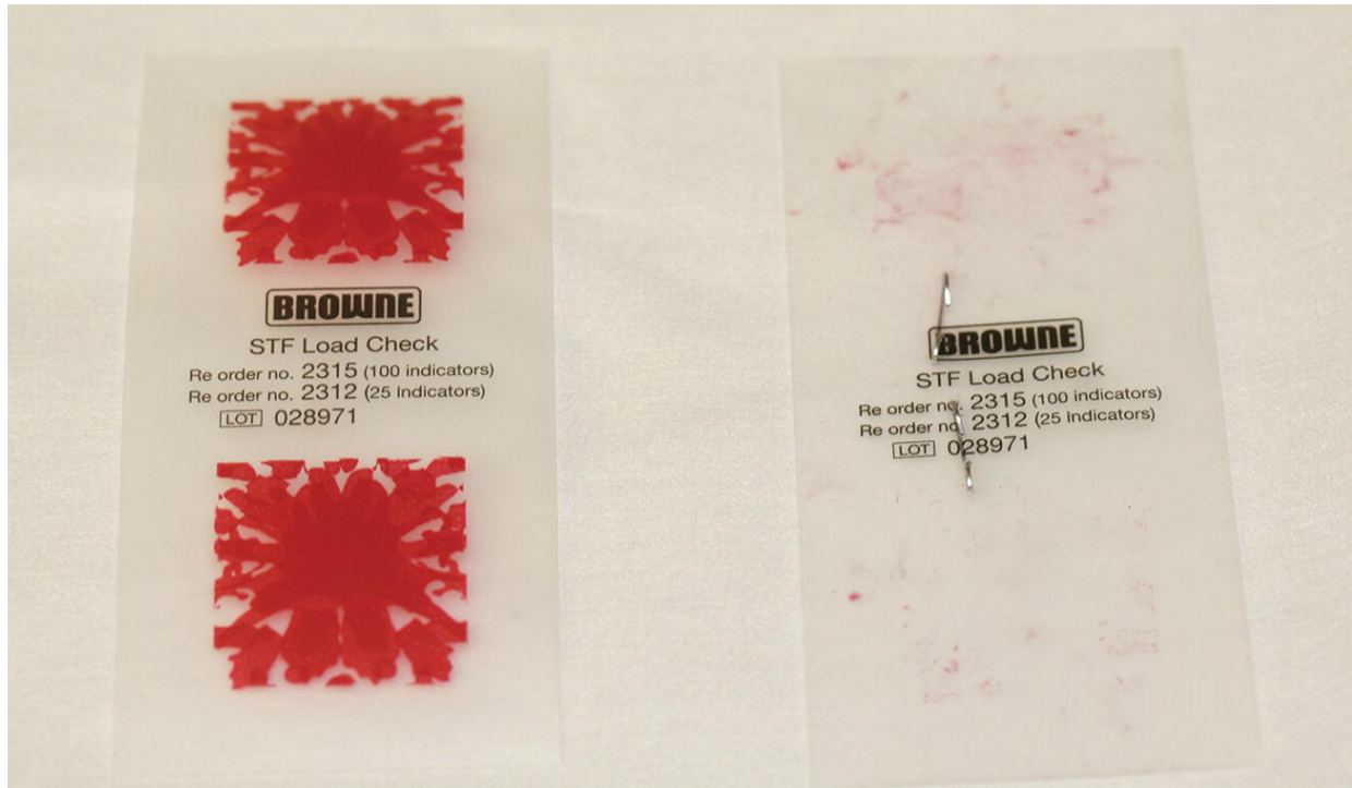
Figure 8.20 Example of 'before' and 'after' test sheets to validate washer-disinfector efficacy.
