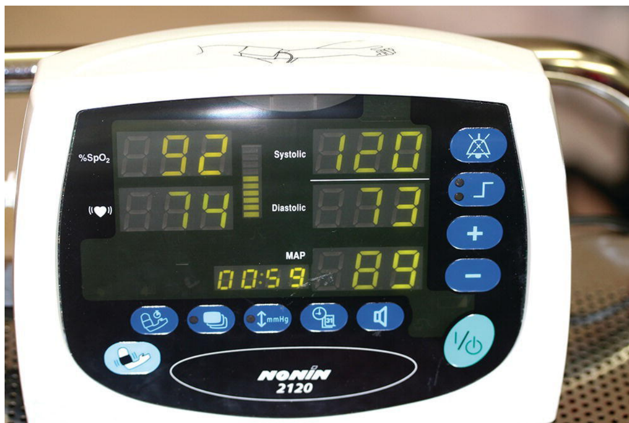
Figure 14.19. Example of a pulse oximeter machine with blood pressure reading facility.
