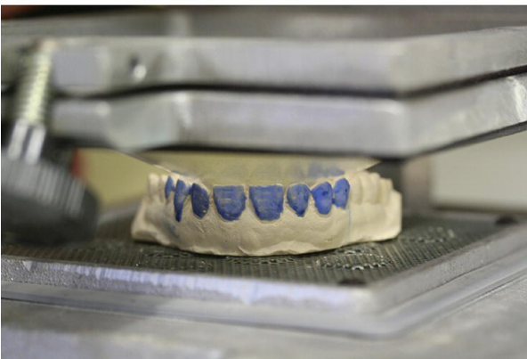
Figure 18.50 (a) Vacuum action as EVA sheet is pulled down onto model. (b) Sheet sucked completely over model to form tray.
